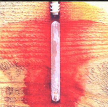
Borate diffusion from Impel Rod
