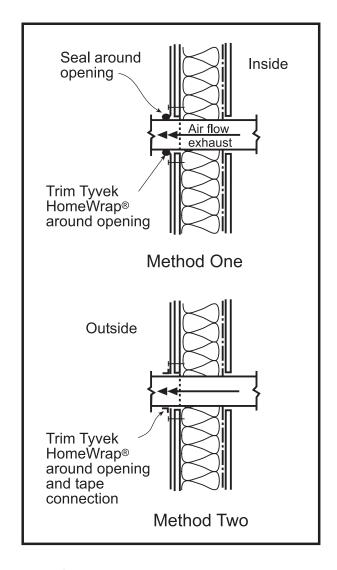
Figure 7. Sealing at wall penetrations.
