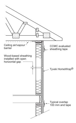
Figure 1. "Tyvek<sup>®</sup> Homewrap<sup>TM</sup>" exterior wall cross-section – top wall/ceiling continuity.
