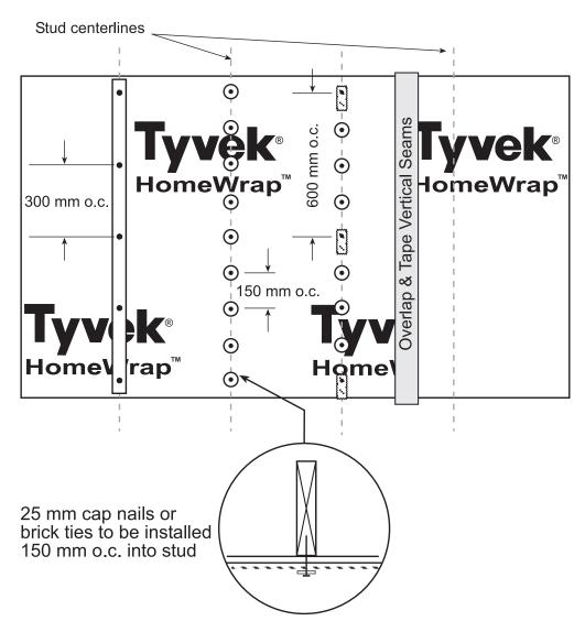
Figure 3. "Tyvek® Homewrap™" structural fasteners.
