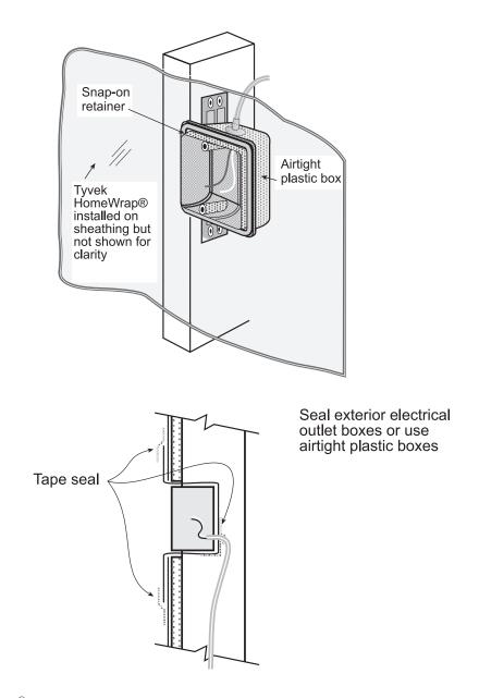
Figure 6. "Tyvek® Homewrap™" exterior electrical boxes.
