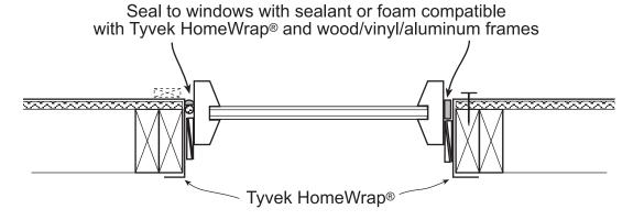
Figure 5. "Tyvek® Homewrap™" window frame cross-section.
