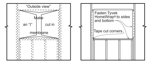
Figure 4. "Tyvek® Homewrap™" window and door openings.
