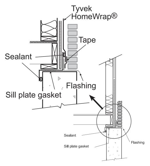
Figure 2. "Tyvek® Homewrap $^{TM}$ " bottom foundation detail.
